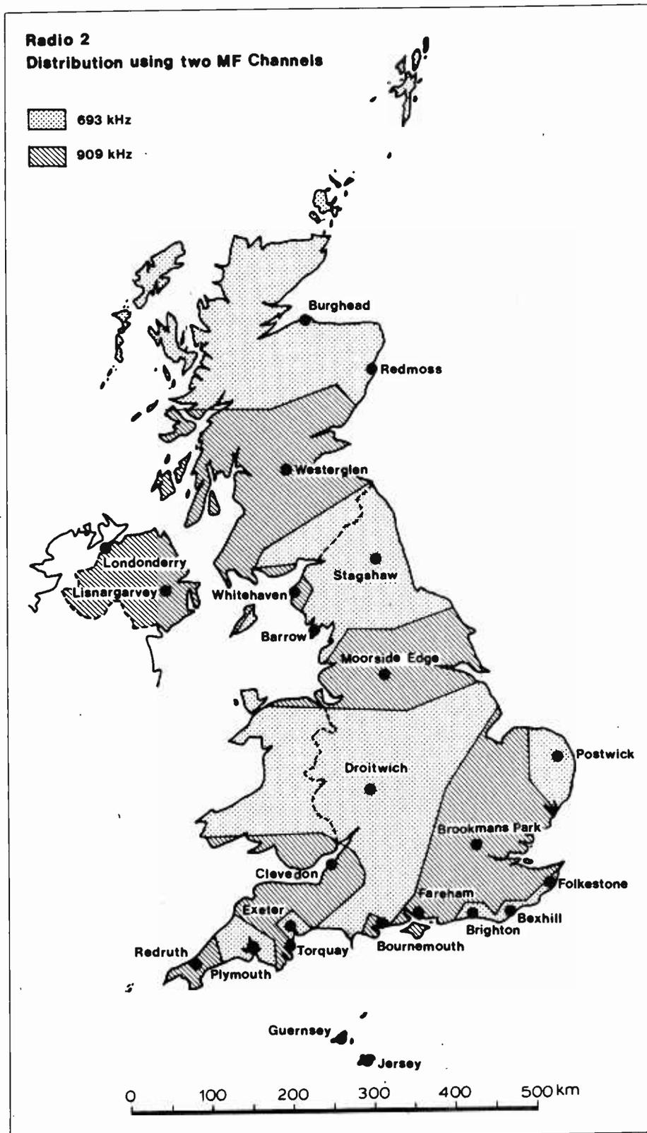
*Radio 2 distribution. The map shows which frequency is most likely to provide satisfactory reception in any particular area. Although a signal should normally be audible in the day-time, the areas of satisfactory reception at night-time will be much more limited than those shown.*
