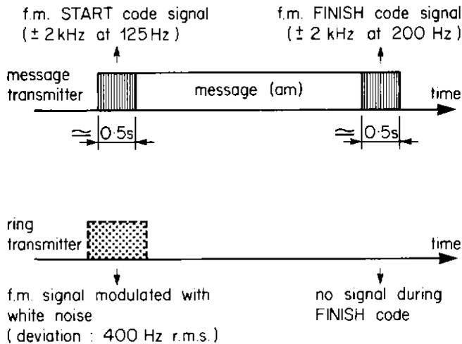
Fig. 3 — Sequence of events in the ring system.
