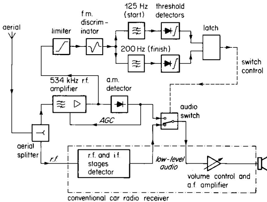
Fig. 4 – Basic features of an integrated receiver.
