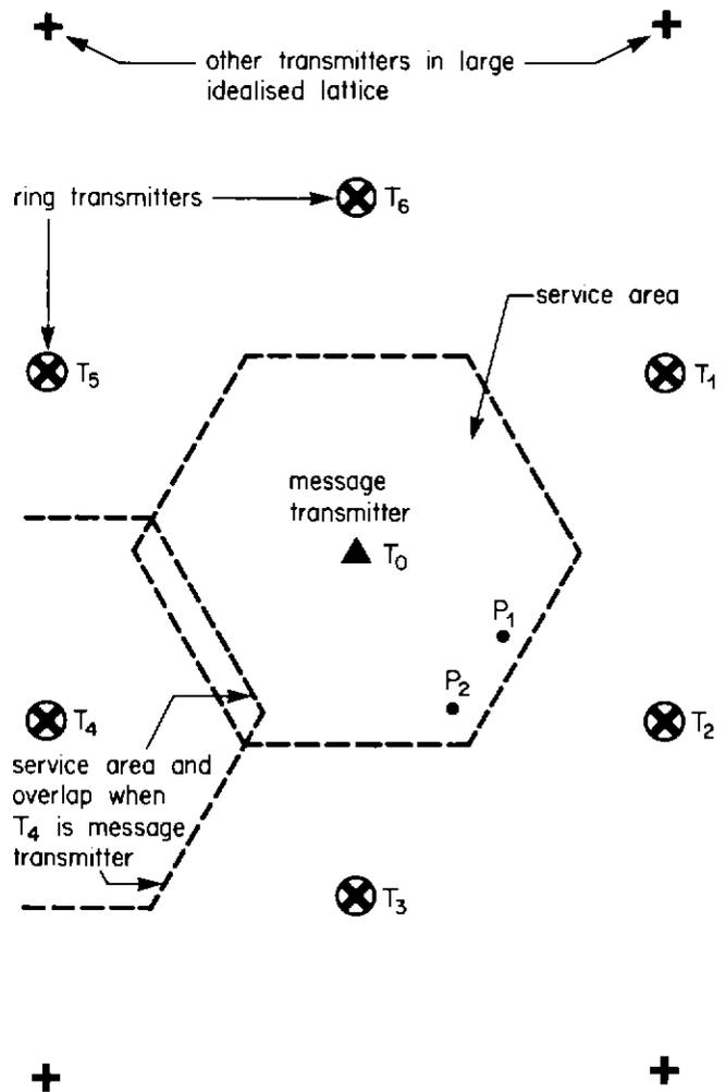
Fig. 2 - Basic arrangement of the ring system.
