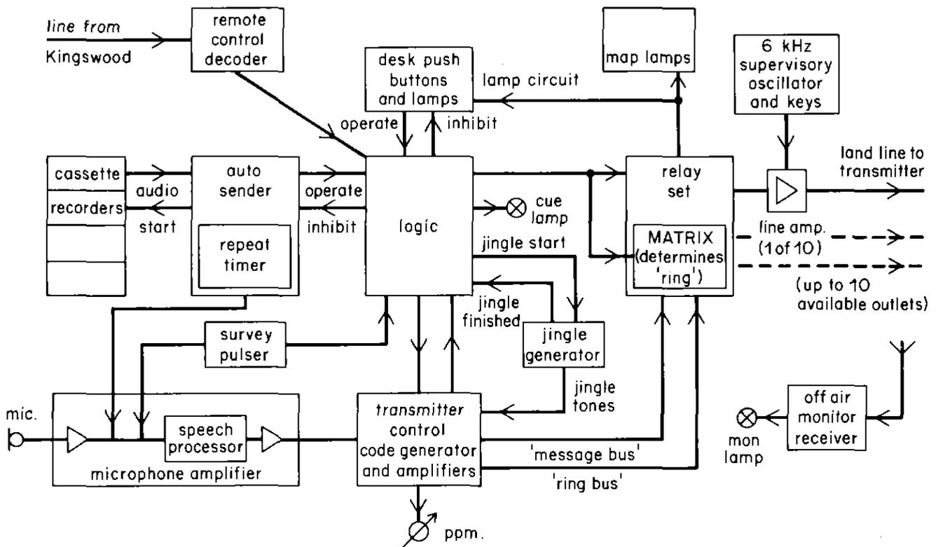
Fig. 6 – Block schematic of the Control desk.
