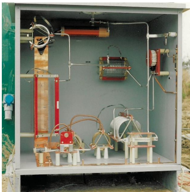
Figure 13. The original aerial matching system Photo: David Thorpe
